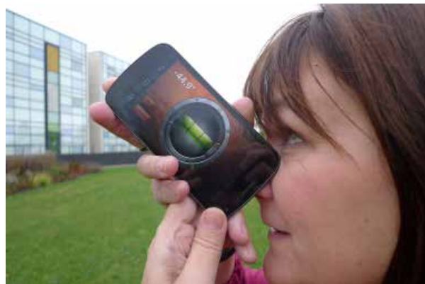
Using a mobile phone tilt sensor to measure the height of a building
